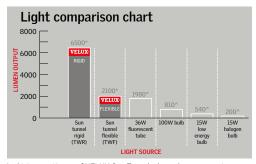
Light transmittance of VELUX Sun Tunnels depends on parameters such as sky conditions (cloudy/sunny), direction of sunlight, orientation and length of Sun Tunnel, VELUX Sun Tunnels in this chart have been tested with a 1 metre shaft, on a 15° roof pitch in summer, at noon on a sunny day using a photometer. (TWR rigid tunnel emits 440 lumens when measured on a cloudy winter's day).
